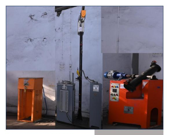
The equipment measures (i) Coke Reactivity Index (CRI) and (ii) Coke Strength after Reaction (CSR), indicative of the performance of coke in the Blast furnace. 200 g of sample is heated with CO<sub>2</sub> at 1100°C in a retort, followed by tumbling. The percentage of mass loss gives CRI, and the percentage of + 10 mm particles retained by tumbling gives CSR as per ASTM protocol. The data is useful in determining coal quality for blast furnace applications.
