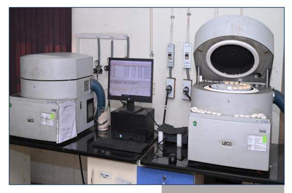
Proximate analyzer is used for proximate The analysis of coal. instrument determines the moisture, Ash, Volatile Matter, and loss on ignition content of coal by measuring the weight loss at different temperatures in controlled environment. 19 samples analyzed can be simultaneously in selectable Nitrogen, Oxygen or Air atmosphere.
