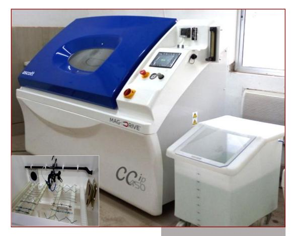
studies То perform corrosion on metals/alloys/nonmetallic materials by means of recreating/accelerating a variety of corrosive climates within the convenience of an enclosed test facility. Facilitates to create 4 distinct climates as follows:
