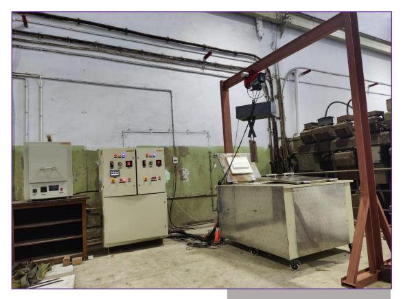
This customized muffle and salt bath furnace setup, equipped with a lifting mechanism, is designed for heat treatment of large-size samples. The muffle furnace can heat samples up to 1100°C, with a 400L × 300W × 450H (mm) heating zone. The salt bath furnace is suitable for interrupted quenching, operating within a temperature range of 200-600°C. It has dimensions of 550L × 450W × 750H (mm) and a salt capacity of about 100 liters.
