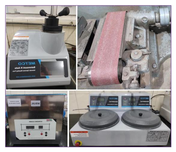
This metallographic sample preparation facility is equipped with various tools, including a belt grinder, mounting press, emery papers and cloths, etching reagents, electropolishing setup, and an ultrasonic cleaner, all designed to prepare a smooth, well-finished surface for microstructural examination.
