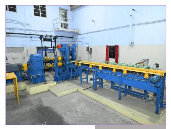
Two high and four high rolling Mill: A two high is for hot rolling and four high rolling mill for cold rolling for ferrous and non ferrous metals, was built by Newfield Engineers Pvt. Ltd. The mill stand has a pair of working roll diameter of 300 mm and roll made of Chilled Cast Iron/Forged with stand hot or cold rolling Mill. Maximum Roll Gap is 70 mm.
