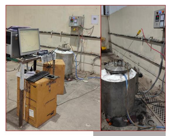
Can be used to examine the corrosion behaviour of the various metal/alloys and coatings in high temperature corrosive environment (especially in molten salt atmosphere).
