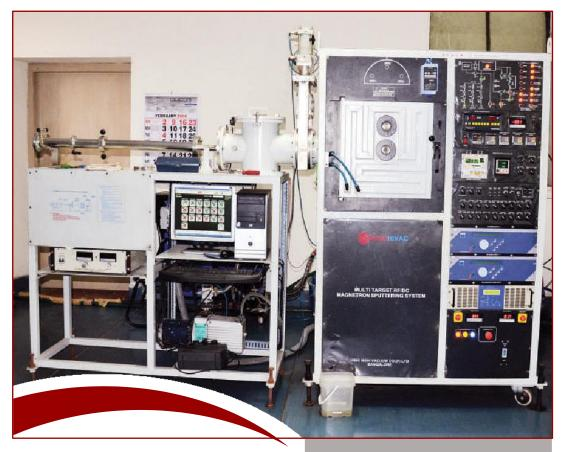
The magnetron sputtering can be used for coating single layer and multilayers of metals, alloys, ceramics, and some hightemperature polymers such as Teflon, etc. It is an atomic deposition PVD process, done by plasma generation. The unit has the capability of 1x10<sup>-6</sup> mbar. It has 3 magnetron sources with a substrate holder having substrate heating and biasing facilities up to 700°C and 200 V, respectively.
