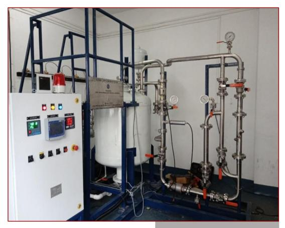
It can be used to simulate the fluid flow and to study the corrosion rate of presence metals/alloys in the of controlled oxygen dissolved in the fluid. The corrosion test rig can be operated/controlled through computer using dedicated software and test data is recorded at set intervals.
