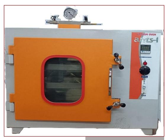
Low temperature heating of any metallic material for the purpose of demoisturizing & structural relaxation.
