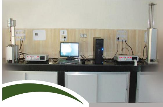
The equipment measures the plastic and dilatation properties of coal on heating as per ASTM protocol. It also measures softening temperature, resolidification temperature, and temperature of maximum fluidity. The data is useful in engineering applications of coal in carbonization, gasification, liquefaction, and combustion.
