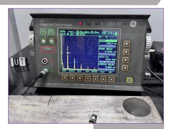
Ultrasonic flaw detector is used to evaluate materials in terms of defects, discontinuities, cracks etc. Various types of elastic modulus can also be determined by evaluating longitudinal and shear wave propagation velocities in materials. Frequency range of the system is up to 25 MHz with a maximum pulser voltage of 450 V. The system is equipped with an analog output port which can be used to save ASCII data for further analysis.
