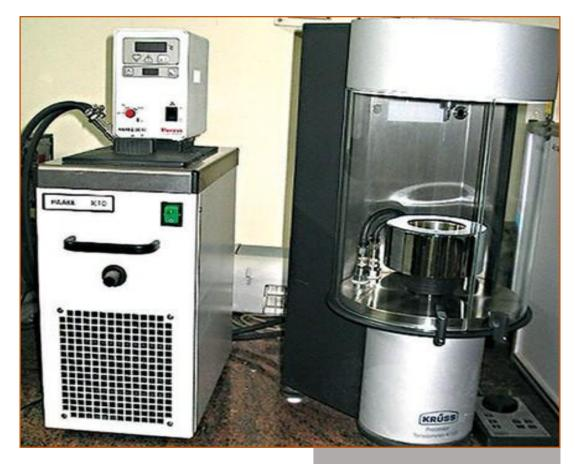
The tensiometer is used to measure the contact angle of solids, powders, and fibre bundles. Surface free energy calculation can be determined from the contact angle data. The surface tension of liquids and, interfacial tension between two liquids can be measured. The measurement method involves both ring and plate (with highly accurate contours) modes of operation. The measurements can be made between temperatures varying from RT to 130°C.
