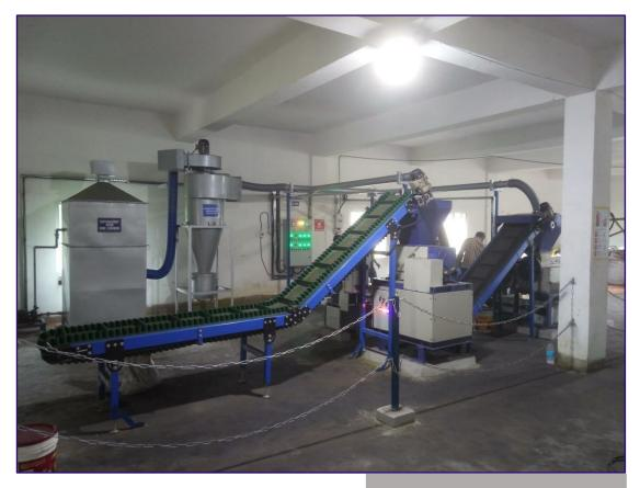
This is a battery dismantling cum processing facility which is capable of processing spent batteries to the tune of 1 ton/day and generates black mass (< 50  $\mu$ m) devoid of copper, aluminium and iron contamination. This facility is available under HOT mode for recyclers and entrepreneurs.
