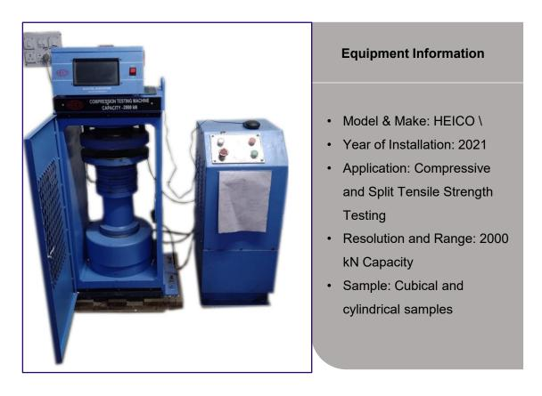
Automatic Compression Testing Machine of 2000 kN useful for measuring compressive strength, split tensile strength.
