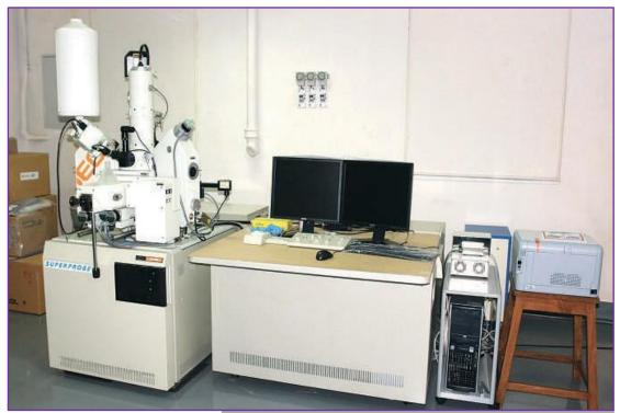
Electron Probe Micro Analyzer (EPMA) is a highresolution elemental analysis instrument combined with wavelength dispersive X-ray spectrometers (WDS) and energy dispersive (EDS) analyzer. It can analyze elements both qualitatively and quantitatively. Depending the on requirement Wand La86 filament can be used. Point, line, and area analyses are possible, also, elemental distribution can be identified by map analysis. The minimum probe size is 0.5 microns (region of analysis).
