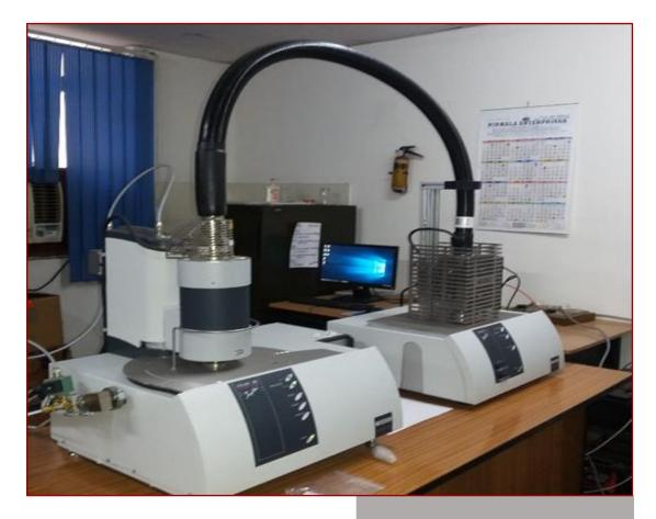
Thermo-Gravimetric Analyzer and Quadruple Mass Spectrometer will be used in studying and characterizing the thermal properties such as mass change, thermal decomposition, evolved gas analysis for a wide variety of samples from minerals to synthesized metal/metal oxide/ polymeric/Organic and inorganic compounds.
