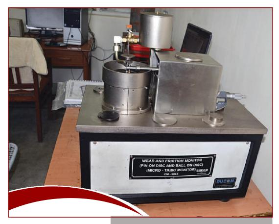
Pin-on-Disc wear tester is used to study the material loss due to frictional forces between the two moving bodies in contact. The system is capable of measuring simultaneously the friction coefficient and wear loss with time or sliding distance under varying load. The lubricability of the fluid can also be evaluated.
