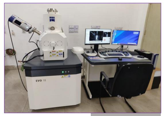
The facility at CSIR-NML is capable of automated imaging and large area composition mapping at a faster acquisition speed. It is a useful tool for quantification of microstructural elements and their composition. Aztec Inclusion Analyzer is custom-designed for acquiring chemical information and identifying inclusions and is capable of classifying as per International standards. aids in the design and control of clean steel production
