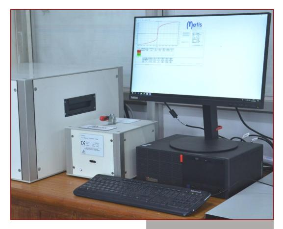
Measurement Platform for the determination of AC magnetic characteristics of soft magnetic materials like soft ribbons & foils.
