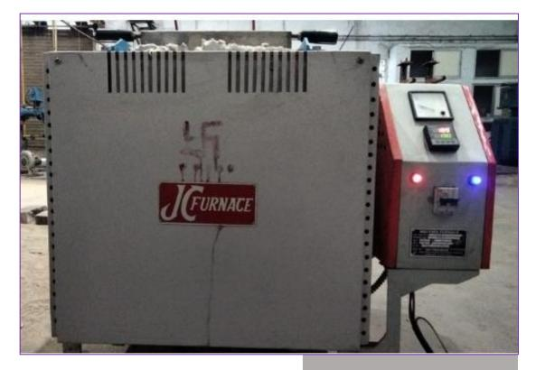
The Aluminum (AI) and Aluminum-Alloys Melting Furnace of 10 Kg capacity is a specialized laboratory apparatus designed for controlled melting and casting of aluminum and its alloys in experimental research. This furnace provides precise temperature regulation, uniform heat distribution, and a stable melting environment, ensuring reproducible results for metallurgical studies.
