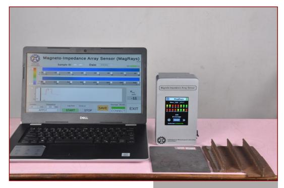
An electromagnetic sensing device based on change in impedance in response to feeble external magnetic field / magnetic phase.
