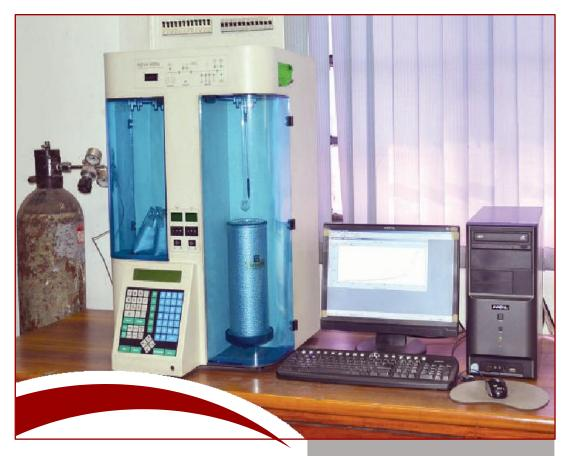
Brunauer-Emmett-Teller (BET) surface area and pore size analysis based on the principle of N, adsorption-desorption method at liquid nitrogen temperature.
