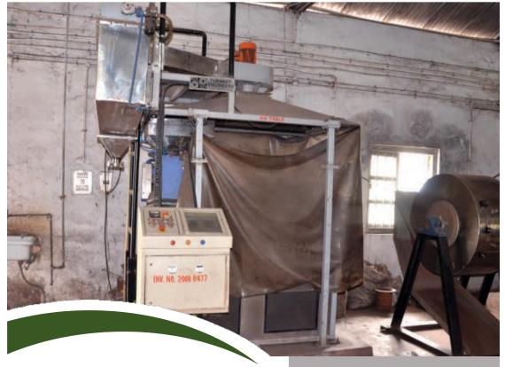
Fluidized Bed Separator/ Air Table is primarily utilized for separation of dry uniformly sized solid particles with differential specific gravity. Air-pulsed fluidization is triggered by air stream and guided into the separating deck. The principle of separation is defined as follows:
