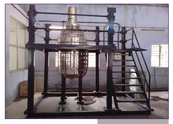
The autoclave is designed for high-pressure leaching operations at optimal temperature conditions. External heating and cooling systems are provided to ensure precise temperature regulation. A heavy-duty motor, powered by a three-phase electrical supply, is integrated to enable rotational movement, promoting uniform mixing and effective leaching. The autoclaves are suitable for carrying out reaction under reducing, oxidizing and inert atmosphere.
