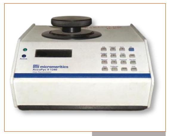
The gas pycnometer is used to measure the true density of the sample by gas (helium) displacement method.
