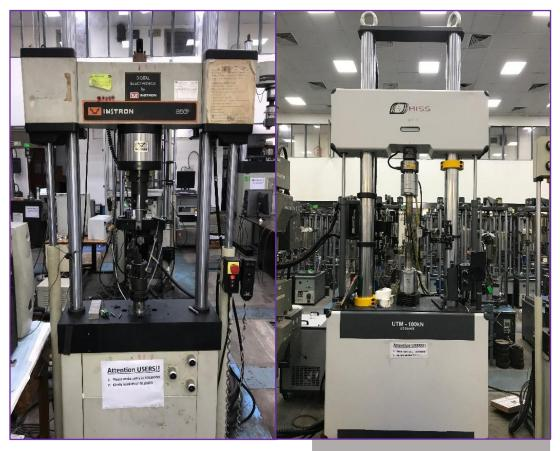
CSIR-NML has 3 numbers of dedicated Creep-Fatigue Test systems of 3.2 T and 10 T capacity with furnace (1100°C) and side entry type high temperature extensometer. The function generator of the system can produce different types of waveforms with long hold time (100 hrs) at either or both peaks.
