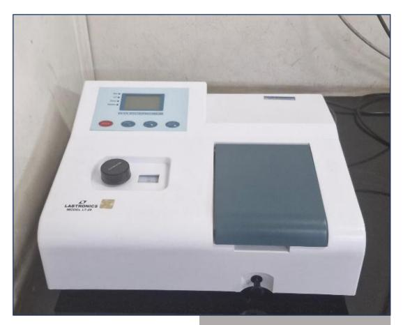
UV-Vis spectroscopy is an analytical technique that measures the amount of discrete wavelengths of UV or visible light absorbed that are by or transmitted through a sample in comparison to a reference or blank sample. This property is influenced by the sample composition, potentially providing information on what is in the sample and at what concentration. The instrument works on the principle of Beer-Lambert law.
