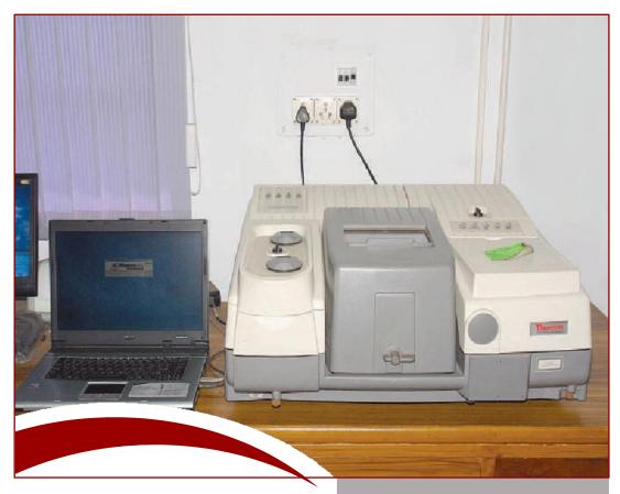
The instrument is useful in detecting the chemical bond vibration of organic and inorganic materials.
