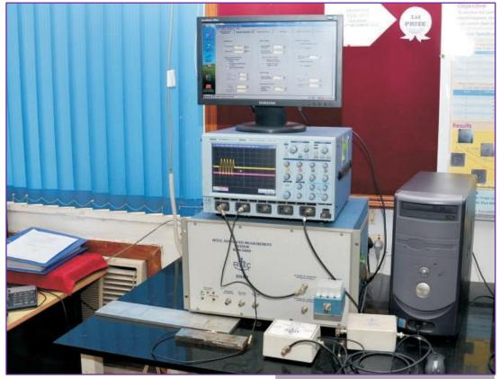
It is a high-power RF tone burst generator with an output of 5 kW up to 7 MHZ. The system operates at a Frequency Range of 40 kHz - 20 MHz. It can be used to characterize material by measuring nonlinear properties. It examines harmonic frequencies for increased sensitivity in material evaluation
