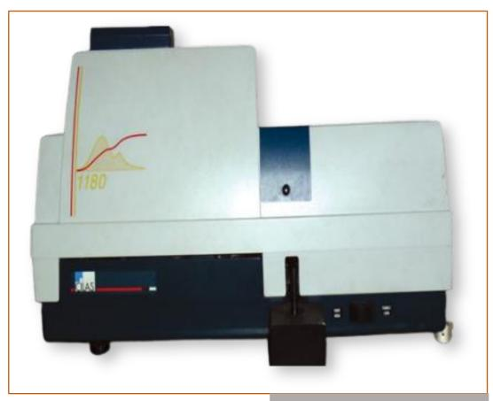
The Laser Particle size analyzer is used to measure the particle size distribution of a sample. It utilizes Helium-Neon laser beam diffraction for the measurement and also considers that the particles are spherical in nature. The analysis involves both dry and wet modes of operation, depending upon the nature and size of the particles. This instrument measures particle size ranging from 0.04 to 2500 µm.
