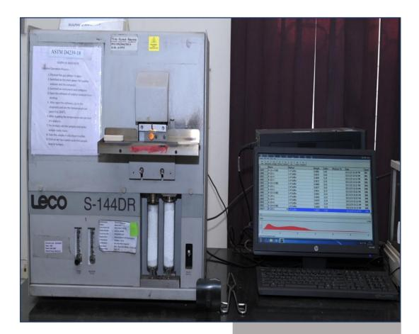
Sulfur analyzer is used to determine total sulfur content in coal. Coal is burnt in presence of excess oxygen and the SO, gas produced is analyzed using IR detector. The analysis is fast with each sample taking 3 min approximately.
