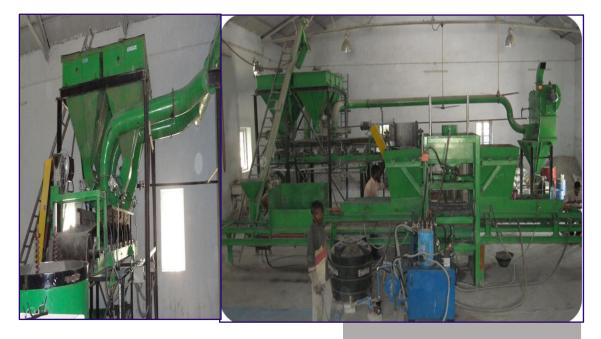
Fully automatic Pilot Plant for block, brick, briquette making
