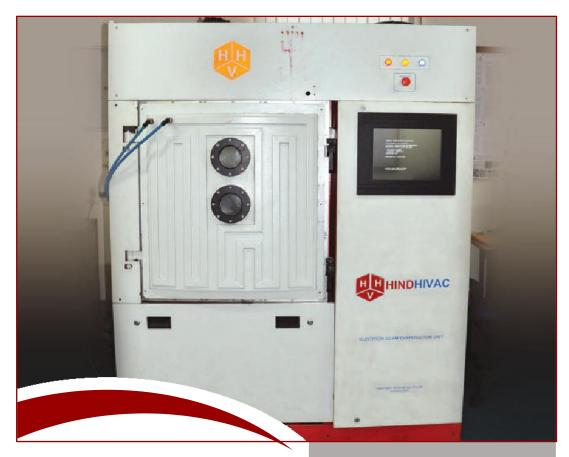
Electron beam evaporation is used for coating single layer and multilayers of metals, alloys, and ceramics. It is an atomic deposition PVD process, done by Thermal evaporation, where the coating material is melted with the help of an electron beam gun. The unit has the capability of  $1 \times 10^{-7}$  mbar. It has 2 electron guns having 4 crucibles in each. The substrate (on which coating is required) also has a heating facility up to 700°C.
