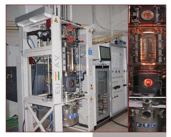
The state-of-the-art national facility, HDPS, can provide a comprehensive solution to industrial issues. It performs a realistic simulation thermal of treatment. galvannealing, galvanizing, and aluminizing processes for Advanced High Strength Steels (AHSS). The optimized parameters directly process can be transferred to the plant for trial.
