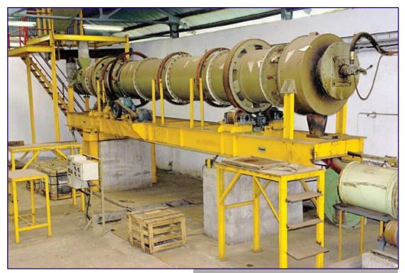
Rotary kiln furnace is operating at 1300-1400°C with a throughput of 100 Kg per hour for calcining the different types of raw materials.
