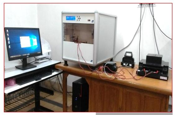
The AC core-loss tester can measure AC magnetic properties for soft-magnetic sheets, strips, powder cores. The setup offers dynamic measurement range between 10 Hz to 200 kHz. The system comprises Epstein frame measurement for Industrial sheets, single strip tester and winding based toroidal core measurements.
