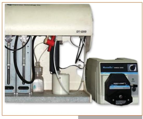
The zeta sizer is a combined acoustic and electroacoustic spectrometer for characterization of particle size and zeta potential of dispersions and emulsions. Zeta potential is determined by measuring colloid vibration current that results from displacement of electrical double - layer of charged particles under influence of ultrasound. The pH range variation is from 0.5 to 13 and particle size measurement ranges from 0.005 µm to 1000 µm.
