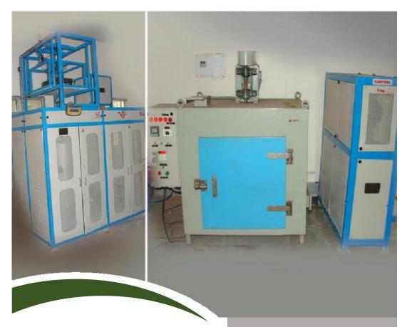
The equipment measures Coke (i) Reactivity Index (CRI) and (ii) Coke Strength after Reaction (CSR), indicative of the performance of coke in the Blast furnace. 200 g of sample is heated with  $CO_2$  at 1100°C in a retort, followed by tumbling. The percentage of mass loss gives CRI, and the percentage of + 10 mm particles retained by tumbling gives CSR as per ASTM protocol. The data is useful in determining coal quality for blast furnace applications.
