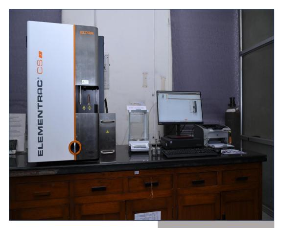
The elemental analyzer ELEMENTRAC CS-i measures the Carbon and Sulfur concentration in predominantly inorganic samples through combustion in an induction furnace and the subsequent analysis of the gaseous combustion products carbon dioxide and sulfur dioxide. The high temperature of more than 2000°C ensures complete decomposition of the sample and thus reliable and accurate elemental analysis over a wide concentration range.
