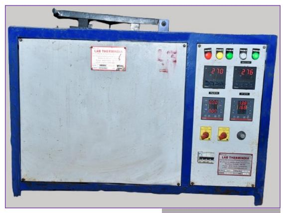
This salt bath furnace offers improved heat transfer to the sample during heating, holding, and cooling cycles, ensuring excellent temperature uniformity across the entire crosssection.
