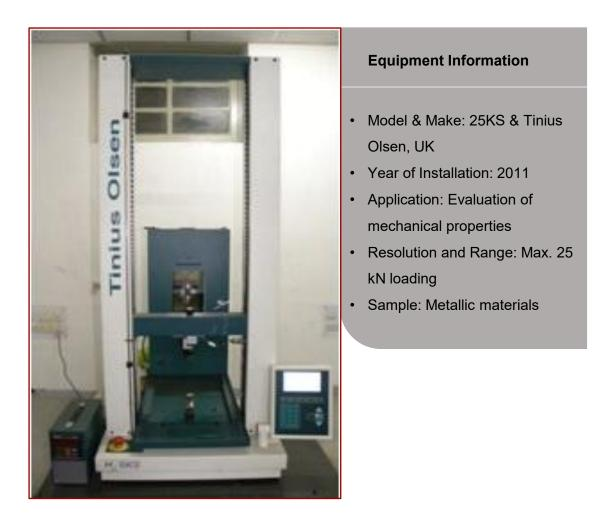
Evaluating mechanical strength and ductility through tensile and compressive testing of metallic samples.
