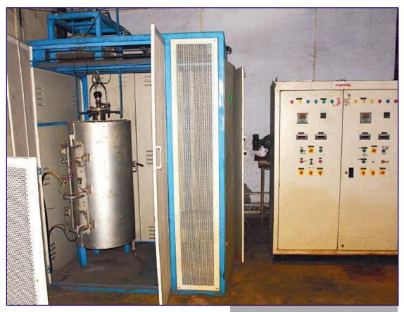
Quality and suitability of using iron ore/agglomerates as iron burden can be estimated prior to its charging in iron making industries. The tests simulate the actual operating conditions.
