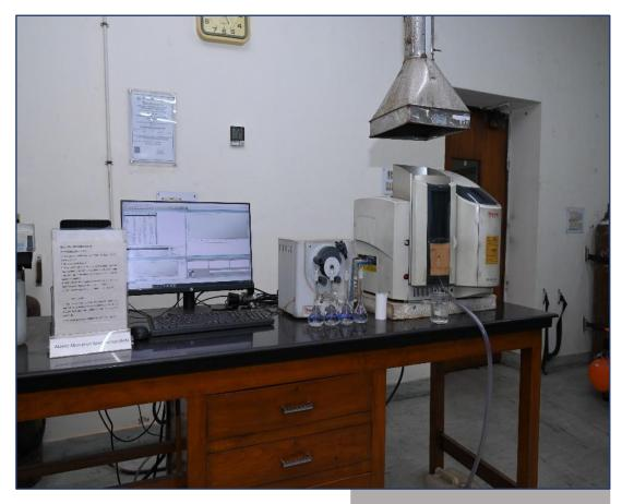
Absorption Spectroscopy (AAS) Atomic detects elements in either liquid or solid samples through the application of characteristics wavelength of electromagnetic radiation from the light source. Individual elements will absorb wavelengths differently and this absorbance are measured against standards.
