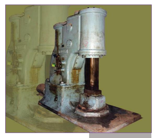
Three Pneumatic power hammers of 1 ton, 0.5 ton and 0.1 ton capacities have been used for open die forging.
