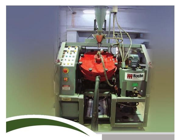
Kelsey Centrifugal Jig is an enhanced gravity separator which allows separation of mineral particles in the fine size ranges. The Kelsey Jig is based on the principles of conventional mineral jig but operates at g-force 100 times that of gravity. This results in improved separation efficiency particularly in fine sizes. The feed particle size to be treated by Kelsey Jig should be < 500 micron.
