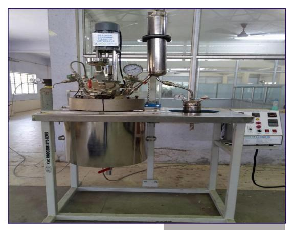
The autoclave is used for high-pressure leaching processes at optimal temperatures. External heating and cooling systems are integrated to maintain precise temperature control during operation. The autoclave is equipped with a heavy-duty motor for rotation, powered by a three-phase electrical supply, enabling uniform mixing and efficient leaching. The capacity, MOC and maximum temperature and pressure limits for the autoclaves are given below:
