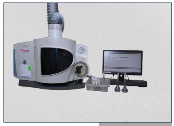
The iCAP7600 series of ICP OES is a powerful dual-view spectrometer, which is used for the analysis of trace, minor & major elements present in aqueous samples like Water, wastewater, leachate, etc. Analysis of Mineral, Ores, Metals, Steel, and other Alloy samples can also be done after their digestion in suitable acid reagents.
