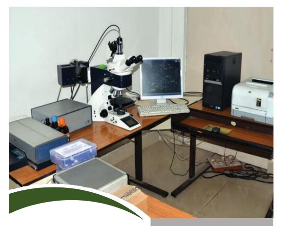
It is the most advanced version of Polarized Light Petrological Microscope, manufactured by M/s Lieca, Germany. It has high-resolution optical devices operating under reflected as well as crosspolarized light modes. Through this, we can have images up to 500 magnification and measure the reflectance/rank of coal macerals as well as have modal counting of macerals and mineral matter on a visual basis.
