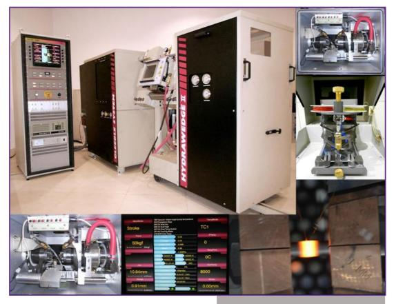
Gleeble 3800<sup>TM</sup> is an advanced experimental system designed for process simulation, material testing and analyzing the thermal behavior of material under different process condition. It can simulate wide range of processes like welding, casting, forming (Hot rolling and extrusion), Heat treatment (Strip Annealing) etc.
